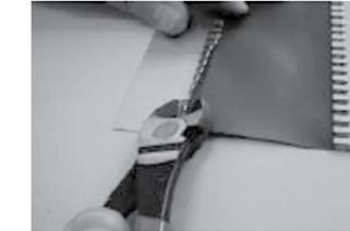
Lift the seam outward to a right angle.
