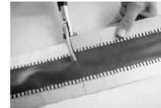
At a notch, cut a length equivalent to the perimeter plus 5 to 6 cm.
