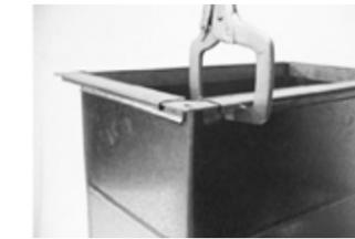
8. Hold SAF - 35 temporarily by clamps until permanent fixing (spot welding or drilling) as shown in next picture.
